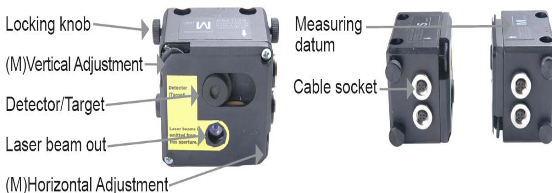
Fig-1a: Transducer front & top view
